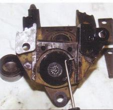
11 Use a pick or other suitable tool to remove both piston seals from their grooves in the caliper.
