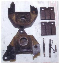
With the bolts removed the caliper will separate. Here's our caliper and constituent parts.
