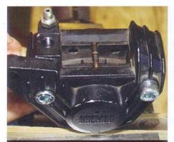
Place the outer caliper half back in the vice and bolt the two halves back together using the supplied new bolts. Reinstall the brake pads and the retaining spring center pin.
