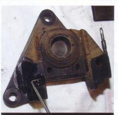
Remove the O-ring seal in the transfer port. It typically stays stuck to the outboard half of the caliper, which has a recess machined into its port to locate the O-ring.
