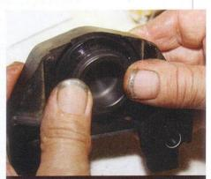
Next, place the new seals into their machined slots in the piston bores (they're cut with square shoulders and will only go in one way), then gently press the pistons into their bores, leaving the top shouldered portion proud of the bore.
