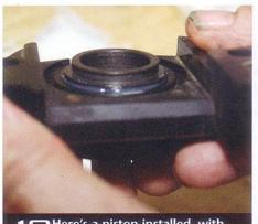
Here's a piston installed, with the shouldered top edge clearly visible. Although not essential, this makes it easier for the next step, installing the dust boots.
