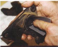
12Clean the caliper halves with brake parts cleaner, then clean off any residual corrosion or contamination using fine-grade Emery cloth lubricated with a bit of brake fluid.
