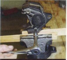
Clamp the caliper by one of its locating lugs in a soft-jawed vice (or use strips of wood to protect the caliper). Remove the two 8mm Allen bolts securing the caliper halves.
