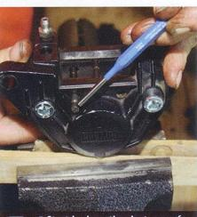
24 Start by inserting just one of the locating pins through the brake pads.
