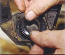
Place the boot over the piston, pressing it into the groove on the piston's shouldered edge. Work your way slowly around and it will push easily into place.
