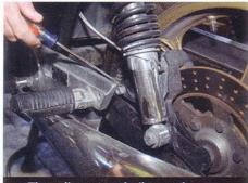
The caliper we rebuilt was the rear unit on editor Backus' 1983 Laverda RGS. It's identical to the front left caliper. Remove the two bolts securing the caliper to its mounting plate. In our case, one of the bolts is obscured by the shock absorber.
