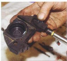
14 With the pistons and bores cleaned up, rinse them thoroughly with brake parts cleaner, then blow out the fluid passages and bores with compressed air.
