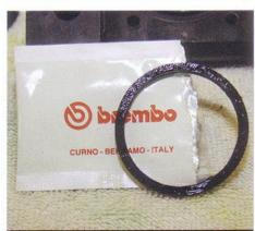
Liberally coat each of the piston seals in a coat of the special brake grease that comes with the kit. Fully compatible with brake fluid, the grease helps ensure easy assembly of the piston into the bore.
