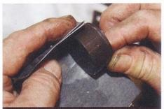
Do the same thing with each piston. We used fine-grade Emery cloth for our initial cleaning, finishing with 1500 grit wet/dry sandpaper. You shouldn't have to be too aggressive, and be prepared to replace the pistons if they won't clean up; deep sanding marks in the pistons will cause the seals to leak.
