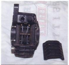
Next, gently pry off the hard plastic brake pad cover. Don't worry if it's missing or breaks while removing; they're readily available.
