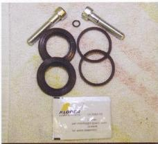
Here's our caliper overhaul kit, containing new caliper halve bolts, the small O-ring for the transfer port, two piston seals, two dust boots and a small package of brake grease.
