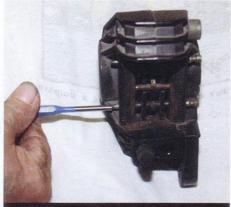
Use a punch to remove the brake pad locating pins, collect the hold-down spring and center spring pin and remove the brake pads. They'll just slide out the top or bottom.
