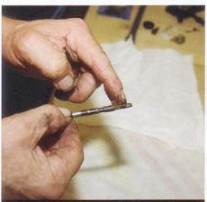
Ensure the brake pad locating pins are straight, then lubricate them with a dab of silicone grease.
