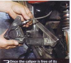
Once the caliper is free of its mount, loosen the brake line, but don't remove it. Instead, hold the line and spin the caliper loose so you don't twist the line.
