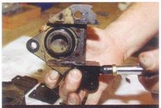
Cover the transfer port with your index finger, then point the piston down against a thick shop rag and blow compressed air through the brake line port to remove the piston. In step #3 we made sure the pistons were proud so we could grip them if they were stuck. Ours weren't.
