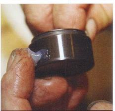
1 Z Likewise, liberally coat each piston and each piston bore with the special brake grease. This picture illustrates nicely how scratch-free our pistons were after cleaning.
