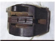
Before we removed the line, however, we applied the rear brake to push the pads in. This will get the caliper pistons proud of their bore and make them easier to remove if the pistons or the bores are dirty or rusty.
