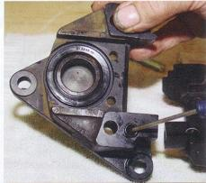
21 Lubricate the new O-ring with brake grease and place it into the recess machined into the transfer port on the outer caliper half.
